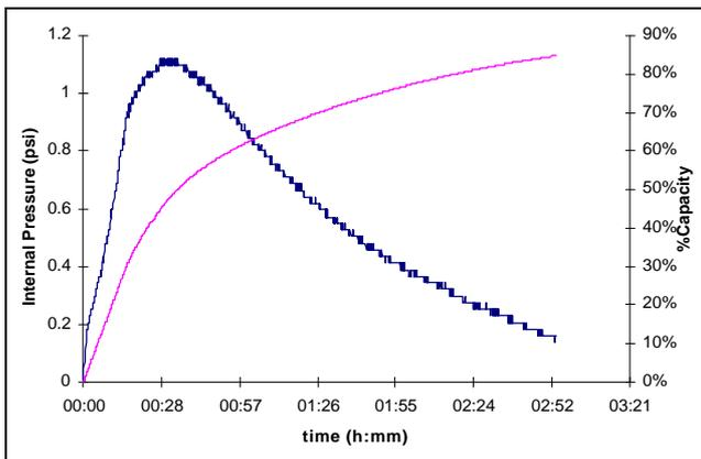
FIGURE 13: Internal battery pressure during pulse charging.
