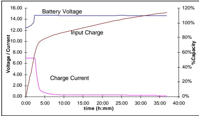
FIGURE 8: Conventional charging of lead acid battery.
