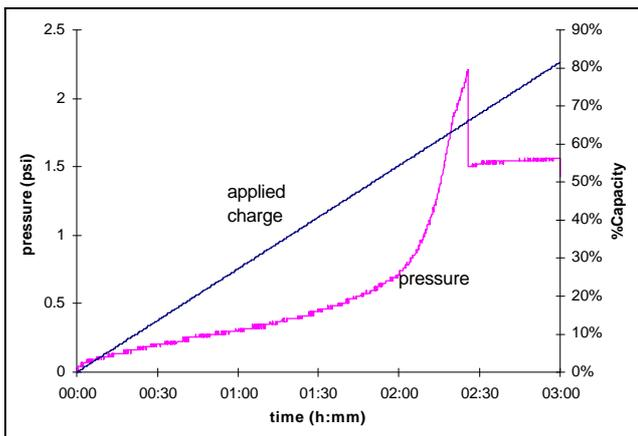
FIGURE 9: Capacity and pressure during invariant pulse charging.
